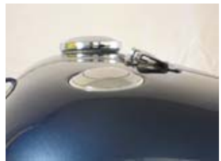
our pop-up gas cap compared with the stock gas cap
