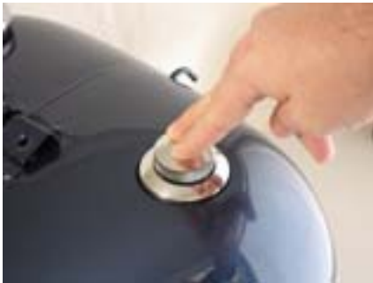
press down the spring loaded center part of our gas cap and rotate it 90 degrees until it locks in position
