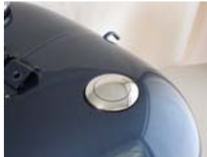
our pop-up gas cap installed
