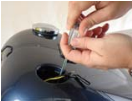
remove the five torx T20 screws with the five coned clear plastic washers (save them because you will need to reuse them)
