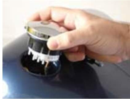
remove stock fuel gauge cap
