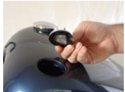
insert the rubber seal underneath our mounting flange. stick the small nipples on the rubber seal inside the small holes on our mounting flange
