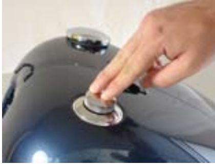
press down the spring loaded center part of our gas cap and rotate it 90 degrees until it locks in position
