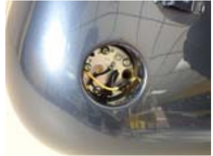
locate the five torx T20 screws
