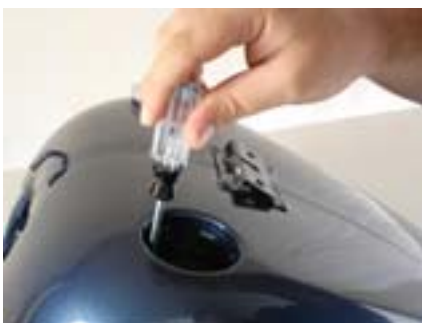
install our mounting flange and stock rubber seal using the five stock torx T20 screws with the five coned clear plastic washers
