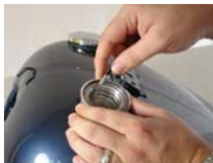
position our gas cap cup on the mounting flange
