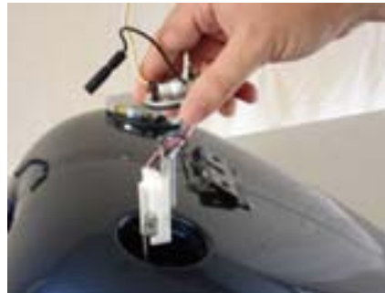
remove the sending unit together with the float
