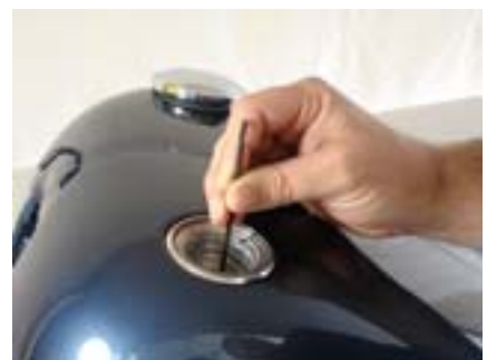
install our gas cap cup on the mounting flange using the three M3 allen screws with lock washers
