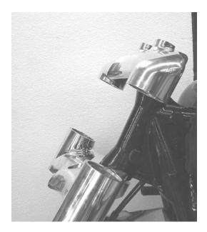
slide steering head bolt through the steering stem. do not tighten yet.
