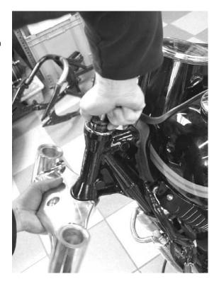
check the steering stem for play in steering head bearings!
